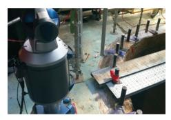
Using a laser tracker, Dimensional Engineering created a world plane and a datum alignment coordinate system. The model accounted for thermal expansion.
