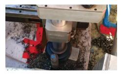
Each sole plate was machined parallel to the Earth's surface and to an elevation within 0.005 of an inch of each plate. It was a level of tolerance that pushed the limits of field machining.
